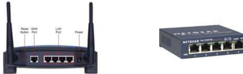
Figure 3 - Wireless Router (left) or Ethernet Switch (right) should be used for hard wired connection.
